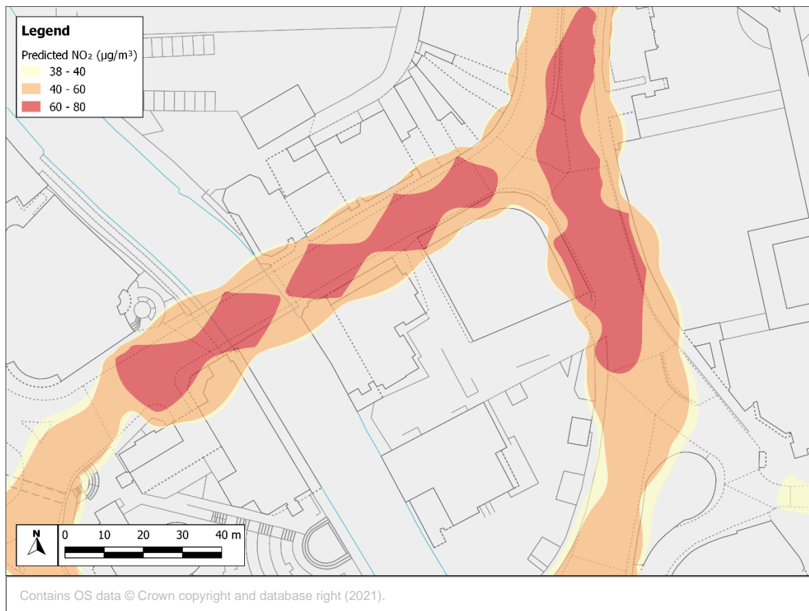
Figure 16: Risk of Exceedance Contour Plot at Gyratory – Bridge Street / Onslow Street
