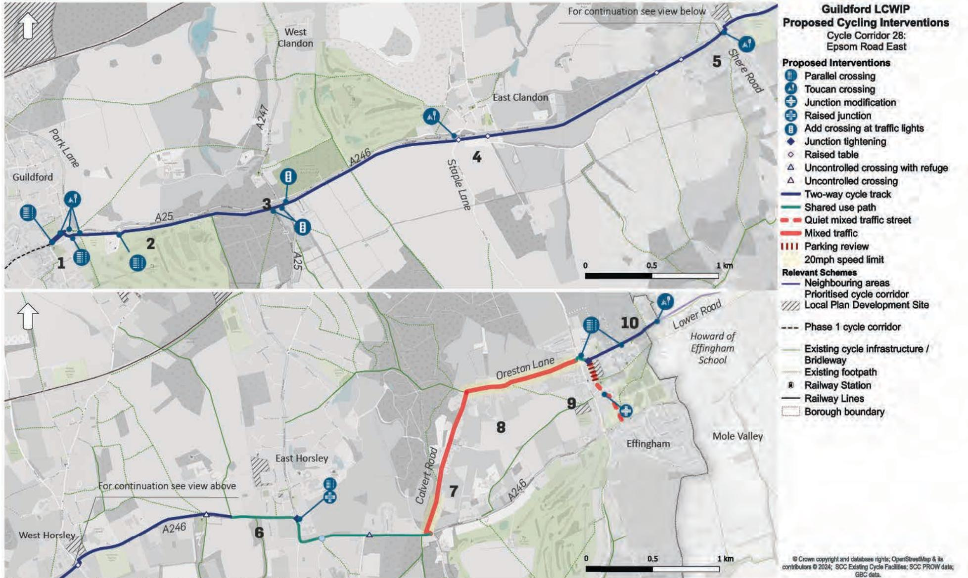
Figure 81. Cycle Corridor 28: Epsom Road East - key interventions
