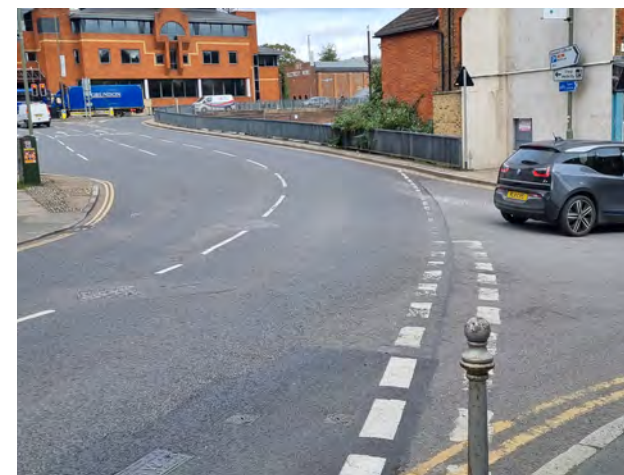
Figure 10. Park Street/ High Street junction: wide bellmouth allows for high turning speeds and limits the space for pedestrians and cyclists.
