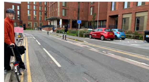
Figure 19. Existing modal filter on Walnut Tree Close allows northbound through traffic and restricts southbound through traffic. Cyclists are permitted bi-directionally. Proposal to restrict all through traffic and allow access only.
