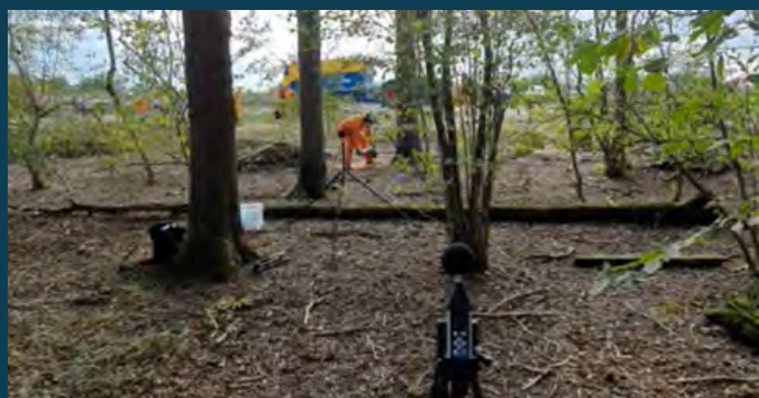
Noise measurement of chainsaw tree felling
