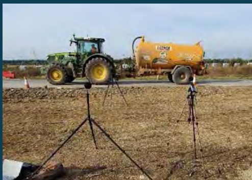
Noise measurement of dust suppression bowser
